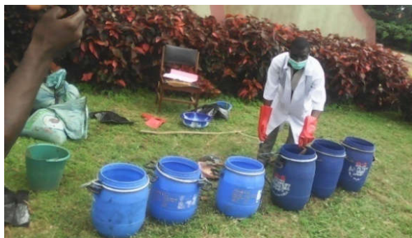
2: Loading of Digester with substrates
