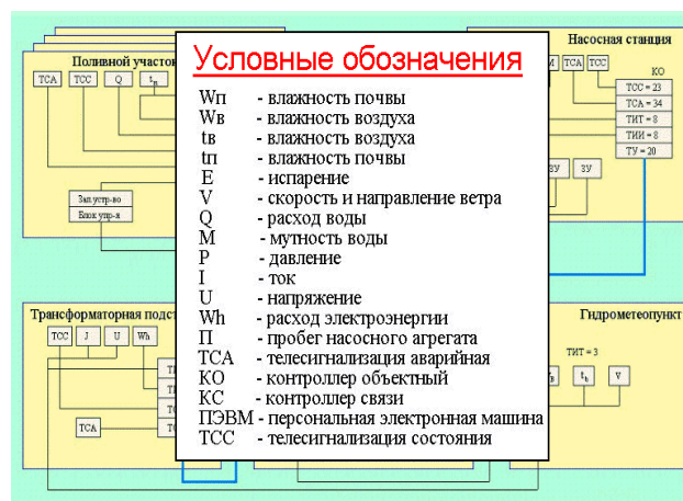
Figure: 5. Structural and functional diagram of the APCS for irrigation
