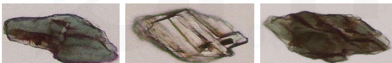
Plate 10. Microscope photomicrography of some heavy minerals represented of the studies soils (Kyanite Green and Kyanite colourless)
