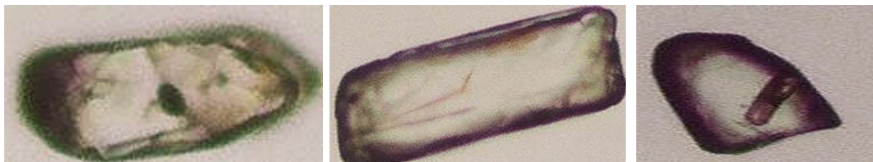
Plate 9. Microscope photomicrography of some heavy minerals represented of the studies soils (Tourmaline colourless Sub angle and angalur)
