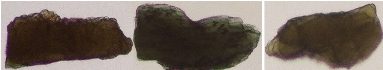
Plate 8. Microscope photomicrography of some heavy minerals represented of the studies soils (Hornblende prismatic dark green and petro chromic Green to pale green).
